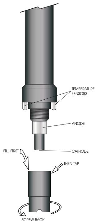
4. Whitt the sensor facing down screw the cap clockwise to the end of the threads. Some electrolyte will overflow.
