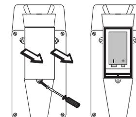
Replacement should take place in a non-hazardous area using a 9V Ni-MH rechargeable battery.
